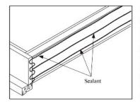
Lay the door unit on edge or face so that the bottom surface of the sill can be caulked. Place very large beads of caulk across the full width of the sill. Additionally, place beads of caulk along the junction of the sill and the jamb and on the bottom surface of the jambs and brickmould.
