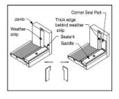
Remove the self-stick paper from the corner seal pads and apply to the door jamb, with the **bottom** lined up evenly with the top of the threshold cap. When the pad is correctly installed, the tab is on top and the narrow part is on the bottom.
