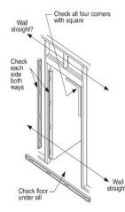
Is the opening the correct size for the door unit? Check it against the door frame size now, before installation. The opening should be frame height plus 1/2 inch, and frame width plus 1/2 inch to 3/4 inch.
